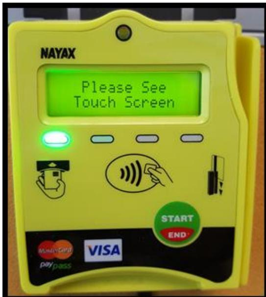
To the left is an example of a machine that has a kiosk that needs to have multiple items selected before **“checking out”** and will not allow a card transaction until pressing a **‘Check Out’** button on the kiosk touch screen display.
