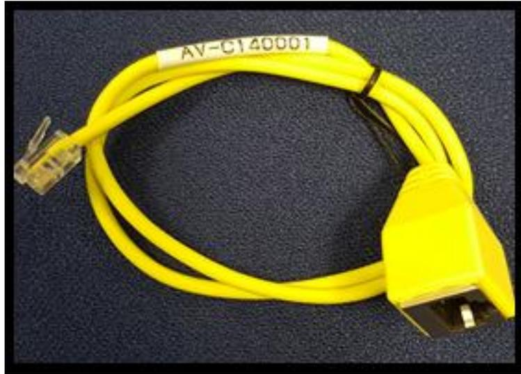
The Vpos Touch ethernet adaptor plugs into the back near the sim card and mdb port. Plug the ethernet cable into this adaptor to use VPOS Touch via ethernet.
