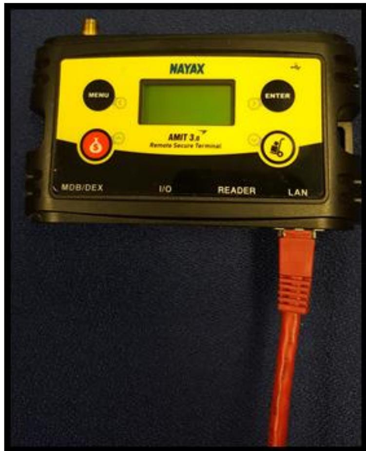
In order to connect a VPOS Touch via ethernet, you will need a separate adaptor called the Vpos Touch Ethernet Adaptor (also called the RJ11 Male to RJ45 Female Cable).
